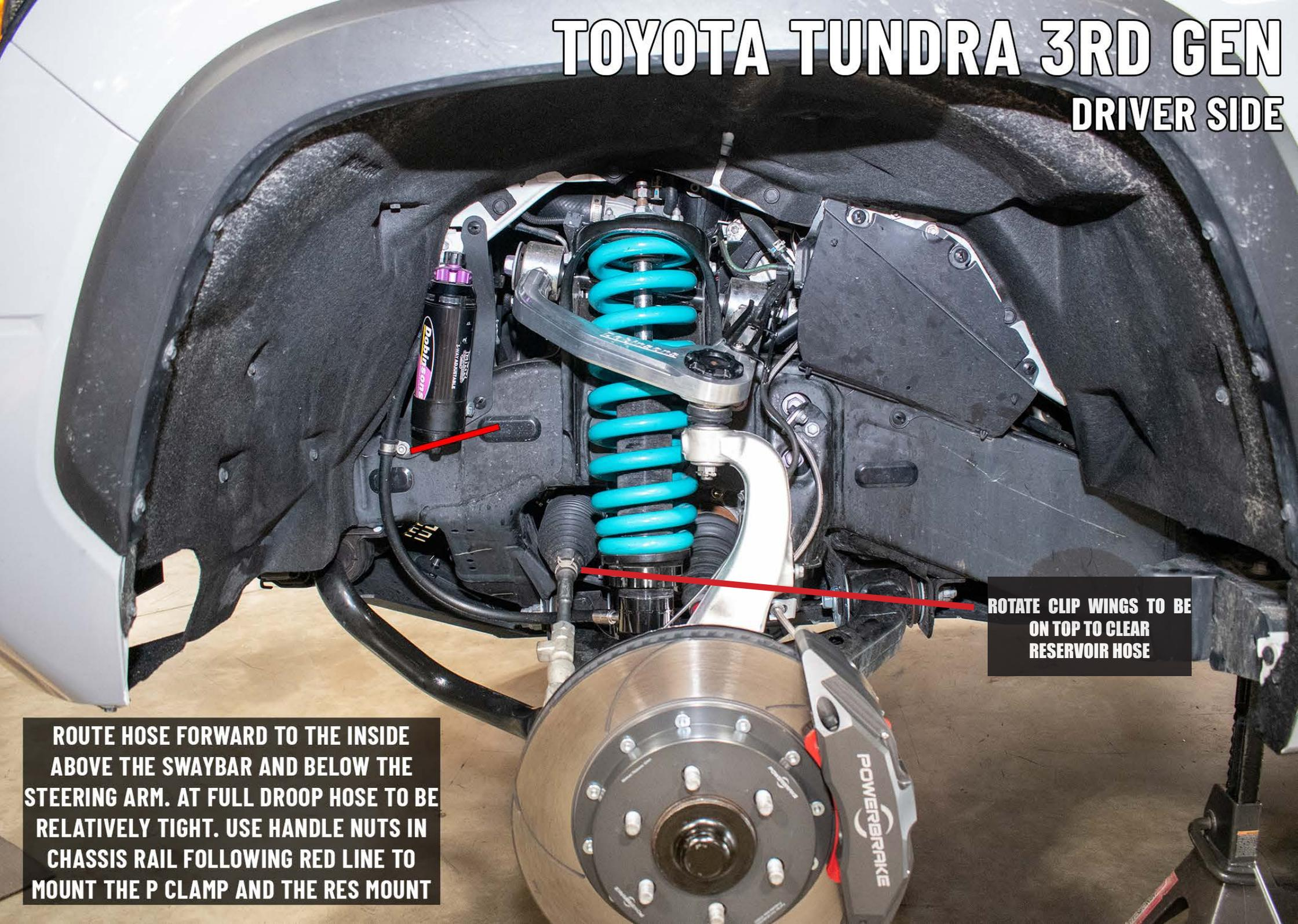
**ROUTE HOSE FORWARD TO THE INSIDE ABOVE THE SWAYBAR AND BELOW THE STEERING ARM. AT FULL DROOP HOSE TO BE RELATIVELY TIGHT. USE HANDLE NUTS IN CHASSIS RAIL FOLLOWING RED LINE TO MOUNT THE P CLAMP AND THE RES MOUNT**
