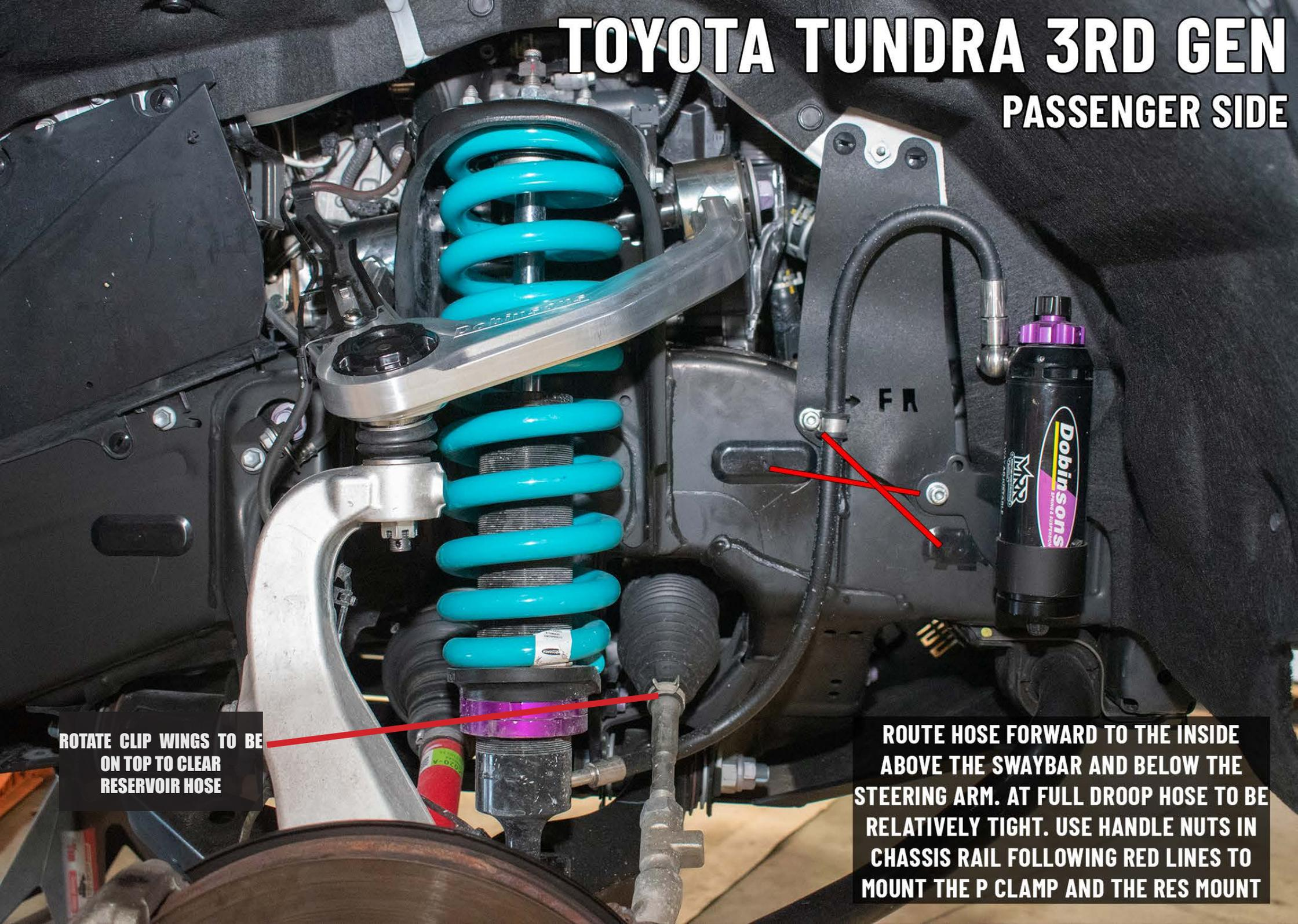
**ROTATE CLIP WINGS TO BE ON TOP TO CLEAR RESERVOIR HOSE**
