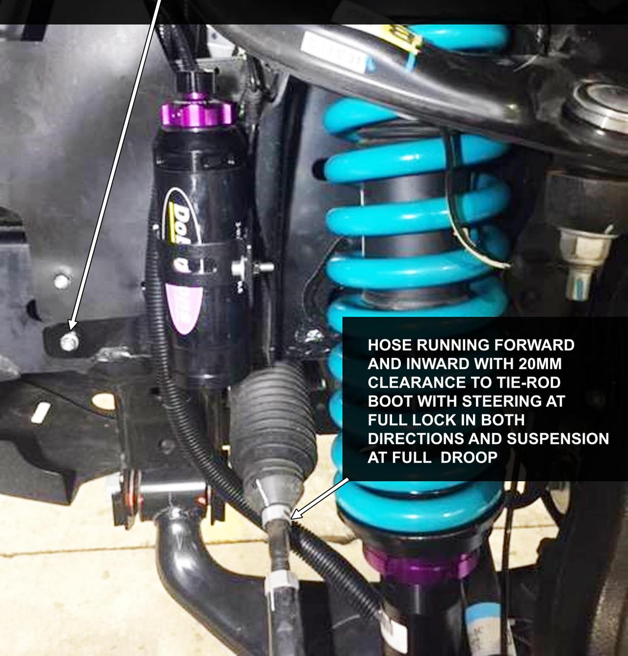
HOSE RUNNING FORWARD AND INWARD WITH 20MM CLEARANCE TO TIE-ROD BOOT WITH STEERING AT FULL LOCK IN BOTH DIRECTIONS AND SUSPENSION AT FULL DROOP
