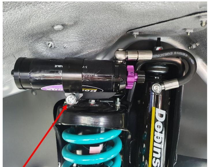
*The reservoir ring clamping block does not need to be overly tight as this may make the shock absorber to firm. It just needs to be tightened until its clamped down then lightly tightened.*
