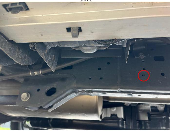
NOTE – If there is no threaded holes you may use the captive nut as per figure 2 to put behind chassis rail and bolt into this. The bolts will then go into this attachment. You may have to bend the chassis nut attachment to get it into the correct position.
