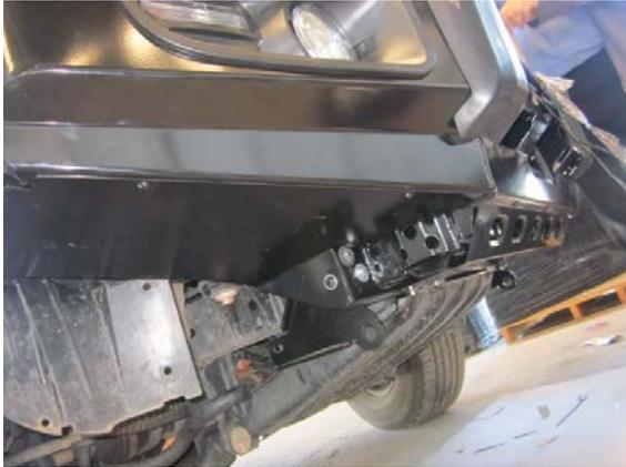
43. Trim the wheel arch mud guard liners level with the bottom under protection kit plates. The captive nuts and bolts supplied can be used to attach the wheel arch liners to the rear of the bullbar.
