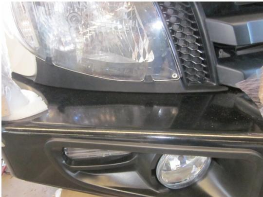
36. Align the bar with the vehicle into its correct position, this will leave about a 10-15mm gap on each side between the bulbar and bottom of the quarter panel, to allow for movement between cab and chassis.
