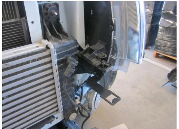
18. Install the LH and RH triangular bracket supports first on the outside of each chassis rails as per page 3 diagram. Insert the captive nut (item 3) through the front of the chassis and insert nuts and washers. The LH bracket can also be bolt at the back.
