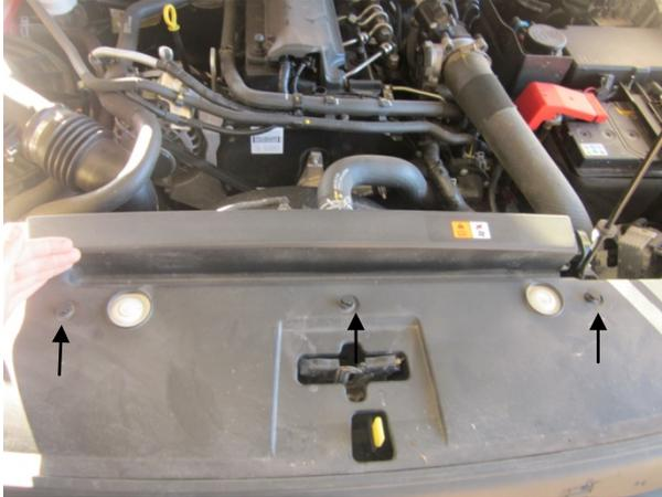
3. Pull the plate upwards slightly and undo the 2 clips underneath holding the top of the grill.
