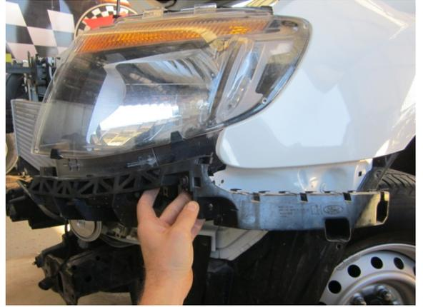
17. Install the New grill support brackets (item 16) onto the spare bolt hole on the inside near the bottom of the headlight, using the 2 x black dome head bolts supplied.
