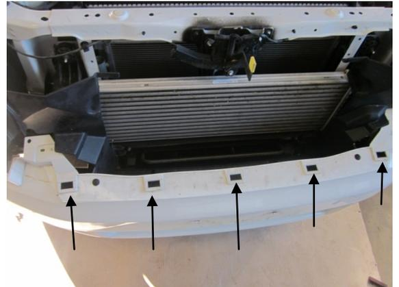
9. Remove all wheel arch liner bolts attaching the wheel arch liner to the bumper, also remove the upper bumper bolt.
