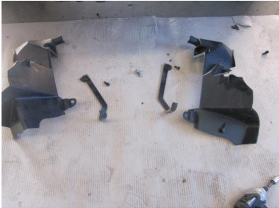
15. Remove the OE bash plate, and keep aside for re-fitment after the bullbar is fitted.
